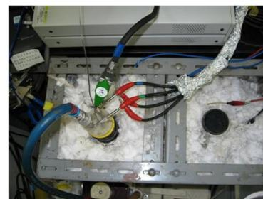
*(Photos Above Left: Impedance analyzer Above Right: looking at the conductivity cell and associated instrumentation)*
